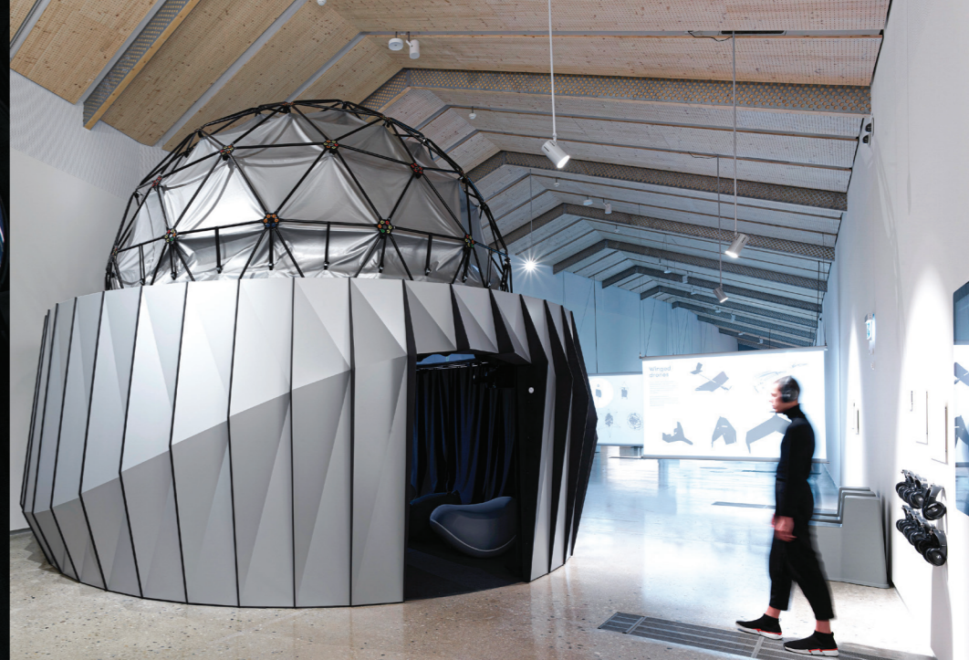
Cupola , one of the Visualization systems at eM+, EPFL. It is a two-projector negative pressure system at 4K, with 5.1 surround sound that can also be used for stereo content. The 4K projector solution uses a cove projection configuration.
