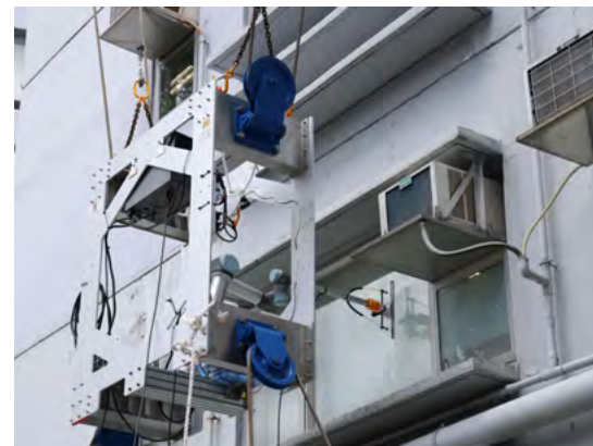
A research team led by Prof. Darwin LAU of the Department of Mechanical and Automation Engineering develops a cable-driven robot which accurately mimics human movement to paint facades and clean building windows
